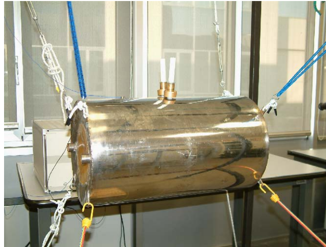
Fig. 1. Experimental shell with two masses with medium rotary inertia.
